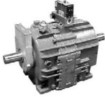
The *Posidyne* Clutch/Brake comes in 9 sizes ranging from Size 02 up to Size 30. The *Posidyne* is the backbone of the Force Control line of Clutch/Brake products. The basic *Posidyne* is a combination of a clutch and a brake in a single totally enclosed unit that is unaffected by outside contaminants and temperatures. An ideal workhorse for the industrial world with a long service life and low maintenance.
