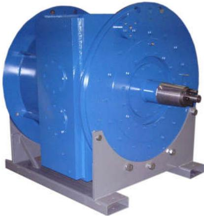
The brake is an “dual purpose” brake. It will control the drop rate during tripping,, absorb the energy from stopping,, and enable stop and hold in position to make the next pipe connection.
